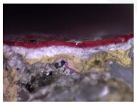
"Niguarda Antifascista" – sample 1 – cross section – reflected Visible light – magnification 35x (left) 150x (right); sample 6: reflected Visible light - magnification 45X Photo credit: ANTARES-CESMAR7
